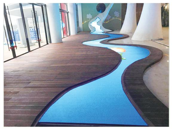
Floor screen are special design for install on the floor and allow people step on it. By integrated with interactive system, it is able to make the contents interactive with the actions for the people who step above the screen.
